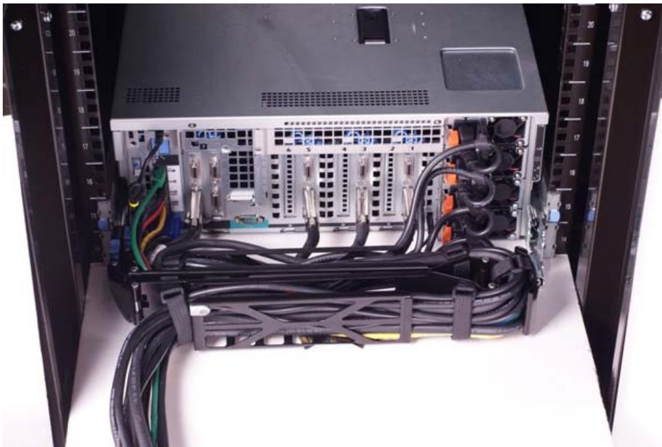
Figure 4: Left-Side Mounted CMA Installation
