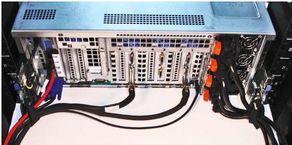
Figure 6: Cable Routing Without a CMA
