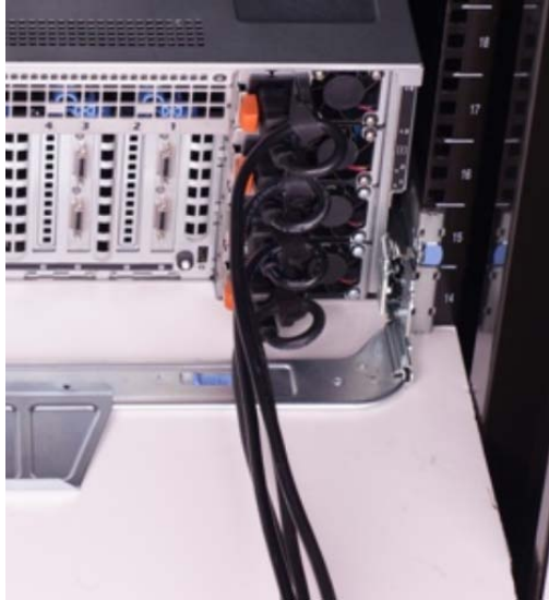
Figure 2: Routing Power Cables Through the Strain Reliefs
